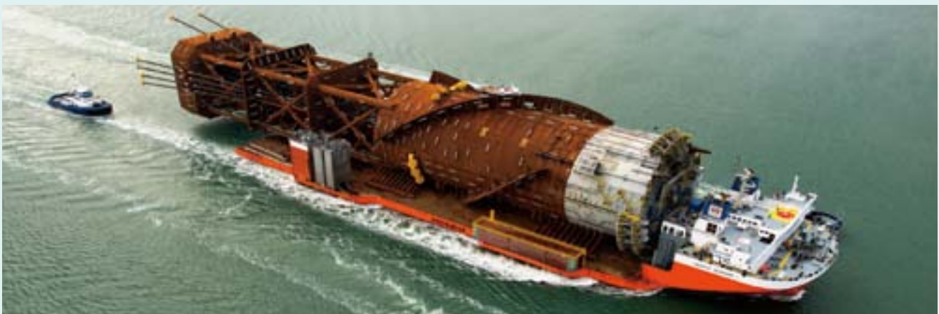
Towing the building frame of a production facility to the development site
