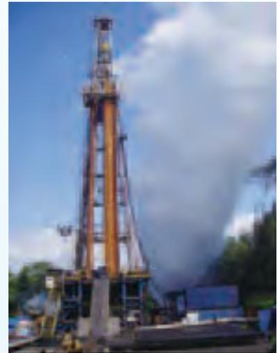
Fumarolic testing at a geothermal well
