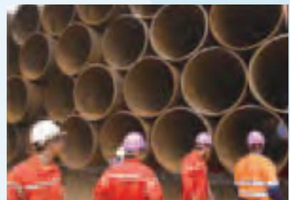
Sections of the 42-inch diameter steel pipes that have been transported to Malaysia for coating
